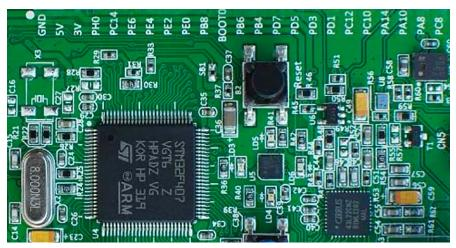
Figure 1: Unnecessary copper GND pour on outer layers.
