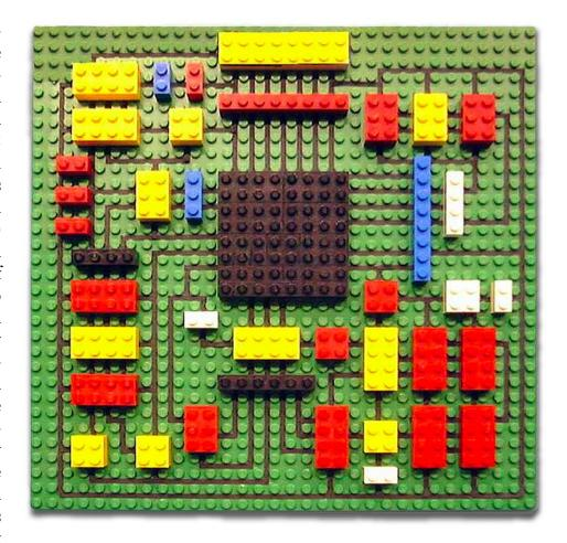
Figure 1: Photo of a mock electronic module created using LEGO bricks in 1995 to visually illustrate the compelling advantage of using components all having standard grid pitch for terminations—making the potential for design layout and routing much simpler.
