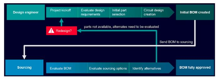
Figure 4: High-level view of the general design and sourcing process.
