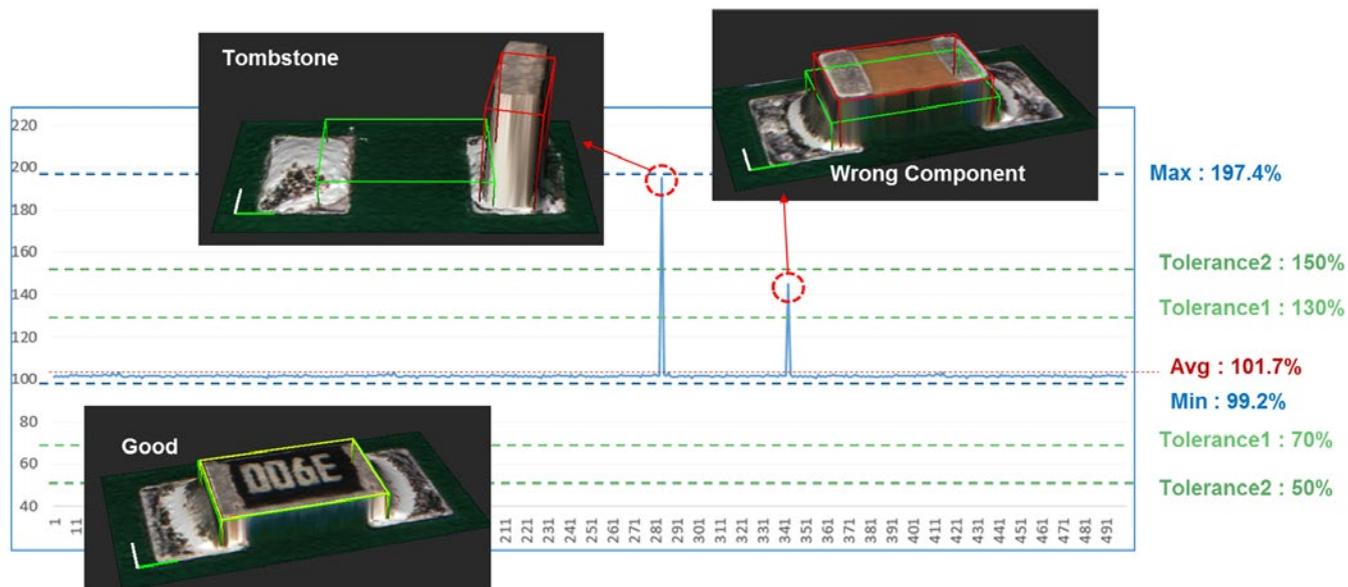
Figure 3: X-bar chart for thickness of R1005 part.
