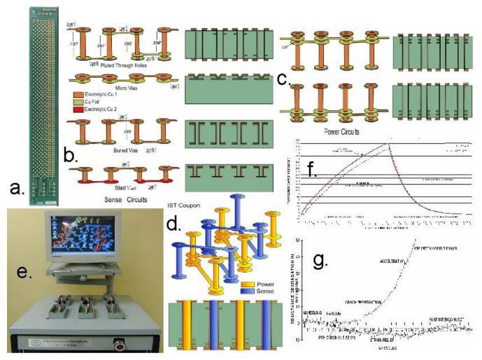
Figure 6: IST is a DC current-induced thermal cycling test; (a) a typical 6" coupon, (b) a sense circuit daisy chain, (c) a power circuit daisy chain, (d) an isometric view of parallel and overlapping power and sense circuits, (e) IST power, data acquisition, and fixturing test equipment, (f) typical heating-cooling cycle, (g) and failure modes of thermally stressed interconnects (PWB Interconnect Solutions Inc., pwbcorp.com) <sup>[5]</sup>.
