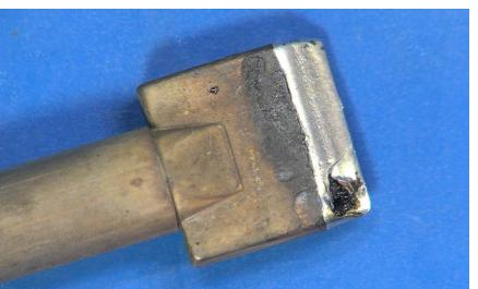
Figure 1: An example of a degraded blade tip.
