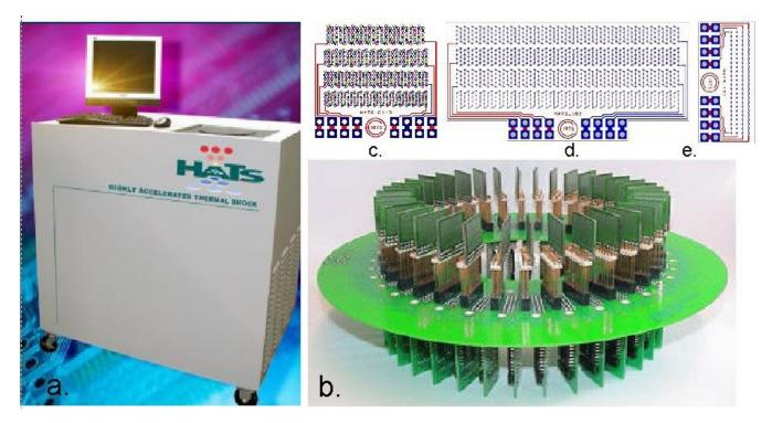
Figure 5: HATS is accomplished by the unit in (a) generating refrigerated and heated air passing over the test fixture (b) that contains 36 test coupons as shown in (c) the 1.0"  $\times$  1.0" or (d) the 2.0"  $\times$  1.0" or (e) the 0.5"  $\times$  1.0" coupons (hats-tester.com) [4].
