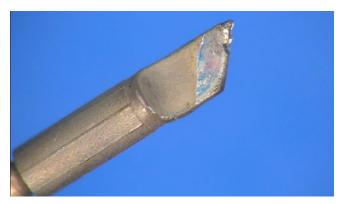
Figure 2: Chisel tip plating erosion.
