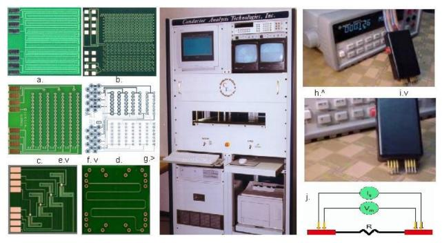
Figure 3: CAT (a) drill overshoot coupon, (b) conductor/spacing coupon, (c) solder mask registration coupon (d) four via nets daisy-chain coupon, (e) impedance coupon, (f) registration coupon, (g) sensitive AC chopped four-wire micro-ohm test system, (h) portable coupon test system using Agilent 34401A meter, (i) close-up of coupon probes, and (j) current and voltage arrangement of the four-wire Kelvin measurement configuration (cat-test.info) [2].
