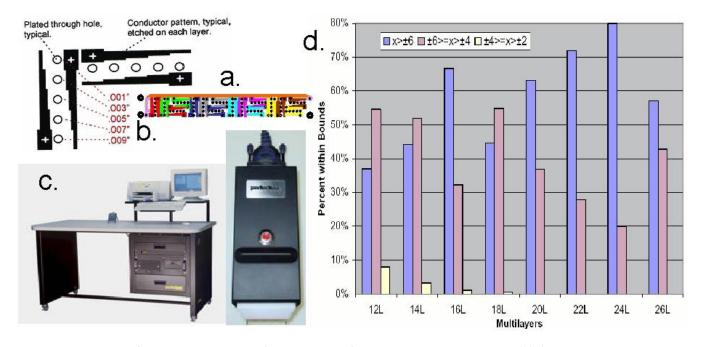
Figure 7: PerfectTest was a material movement and registration coupon system; (a) the coupons were 0.2" x 1.73" and placed at the edges of production multilayer panels, (b) it worked by measuring the continuity of PTH versus the metal foil of specific layers, (c) the testing equipment included a close-up of the probe head, and (d) data from one user in production of nearly 250,000 readings for 12-layer to 26-layer multilayers <sup>[6]</sup>.
