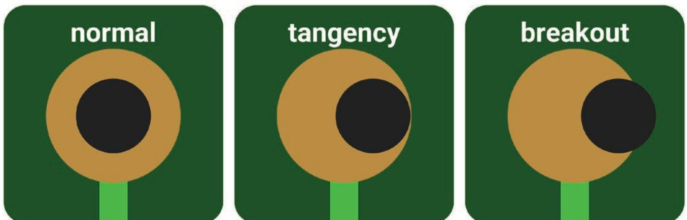
Figure 2: Example of annular ring that is too small.
