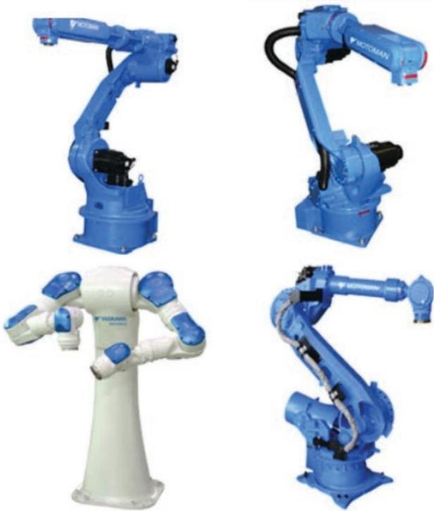
Figure 4: Articulating robotic arms provide racking and panel handling. (Source: Ludy)
