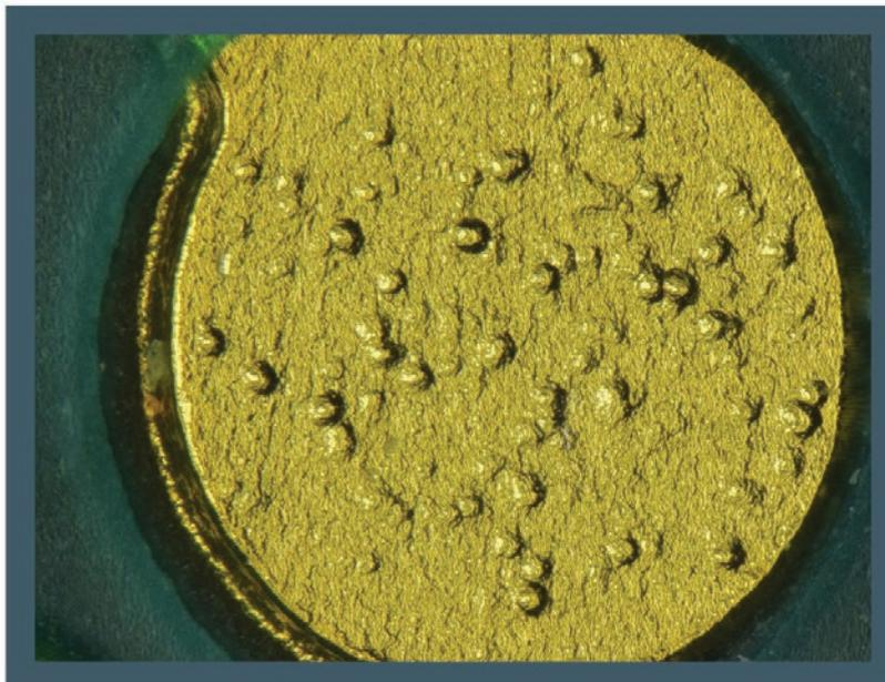
Figure 2: Rough spots due to poor leveling of the copper.
