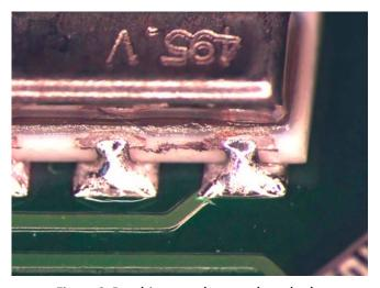
Figure 8: Dendrite growth on package body.
