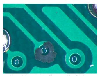
Figure 5: Corrosion in solder mask with pinholes.
