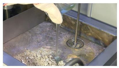
MS2® molten solder surfactant being poured onto the surface of the solder bath.
