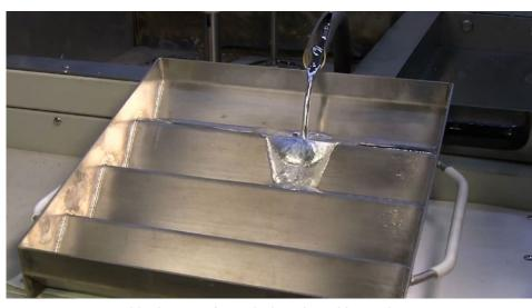
Pure solder bars are formed when the solder cools.
