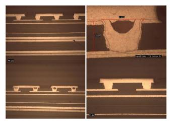
Figure 15: Example of WMI failure caught by OM testing.
