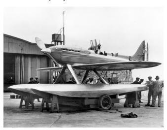
The Supermarine S.6B 1596 seaplane that broke the world airspeed record of over 400 mph. (Source: Wikimedia Commons)
